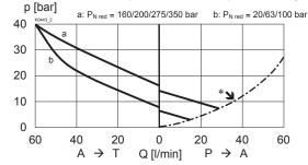
$Q_{st+L} = f(p)$  Pilot- and leakage volume flow characteristic [A (1)  $\rightarrow$  T (3)] (Pressure in P (2) = 350 bar)
