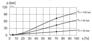
$p_{red} = f(I)$ Pressure adjustment characteristics [at Q = 0 l/min]/(s corresponds to preset value signal) Inlet pressure: p<sub>N</sub> +10 % Mesured with closed port A
