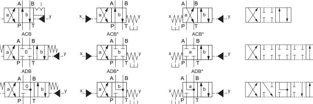
\* These 4/2-way valves with spring reset are being delivered as 4/3-way valves.
