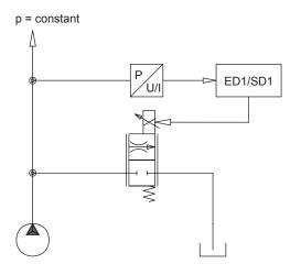
Pressure reducing control with throttle valves (2-solenoid application)
