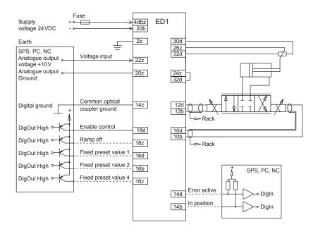
The example shows the controller with 10-Bit analogue inputs connected to a PLC. The programed position is issued by the PLC as a voltage signal. The cylinder actual position is fed back to the controller in the form of a voltage signal of corresponding size.
