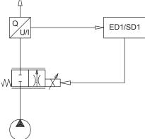
With this system, high dynamic and static requests can be performed. Any proportional valve with one active control edge can be used.
