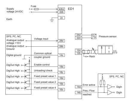
The example shows the controller as a pressure reducing control with throttle valves with 10-Bit analogue inputs (2-solenoid application). The preset value is issued by the PLC as a voltage signal. The actual value is fed back to the controller in the forme of a voltage signal of corresponding size.
