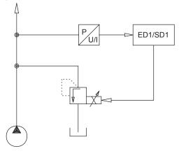
This system is actually only a electronically preset value re-lead. The problem is that the pressure already is mechanical controlled inside the valve. Because this mechanical control is very slow, the electronically control must be made slow artificially (cascade control: the exterior loop must be slower than the interior loop). With such a system, good static requests can be performed. However, dynamic requests can be badly performed.
