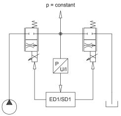
Pressure reducing control with throttle valves for clamping function (2-solenoid application)
