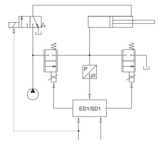
With this system, high dynamic and static requests can be performed. Any proportional valve with one active control edge can be used.
