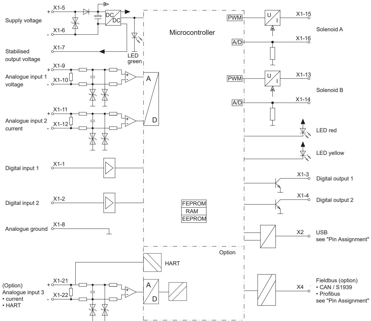
**Configuration Analog inputs Basic amplifier**
