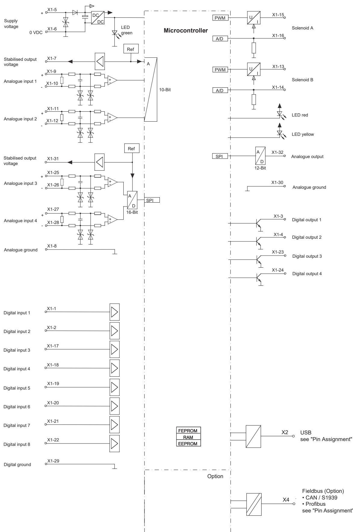
**BLOCK DIAGRAM ENHANCED AMPLIFIER WITH HART**
