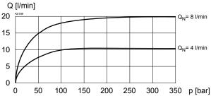
$\Delta p = f(Q)$  Pressure loss/flow characteristics (s = 100 %) [Type: V4D42]
