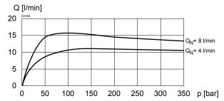
$\Delta p = f(Q)$  Pressure loss/flow characteristics (s = 100 %) [Type: S4D41]
